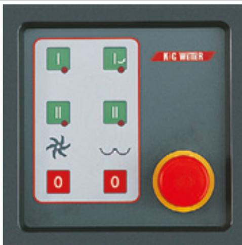
Bowl cutter 33 L, type 425. Operation via foil keyboard (T2). Knife shaft and bowl can be driven at two speeds each.
